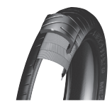
BELTED TYRE WITH RADIAL CARCASS (90 DEGREES)
